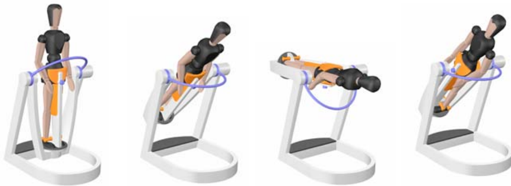
Figure 1: Operation mode of the device for whole body tilt. In contrast to this schematic demonstration for standard applications, during the actual investigation arms were held crossed against chest.
